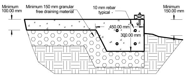
Foundations for detached garages and accessory buildings over 55 m<sup>2</sup> (592 ft<sup>2</sup>), but not greater than 70 m<sup>2</sup> (753 ft<sup>2</sup>), in building area with a rafter/roof truss span no greater than 10 m (33 ft) may be placed on the a foundation conforming to the following specifications.
