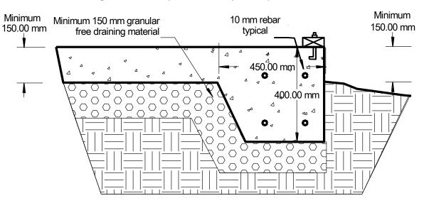
Foundations for detached garages and accessory buildings over  $70 \text{ m}^2$  (753 ft²), but not greater than  $100 \text{ m}^2$  (1,076 ft²), in building area with a rafter/roof truss span no greater than 10 m (33 ft) may be placed on the a foundation conforming to the following specifications.
