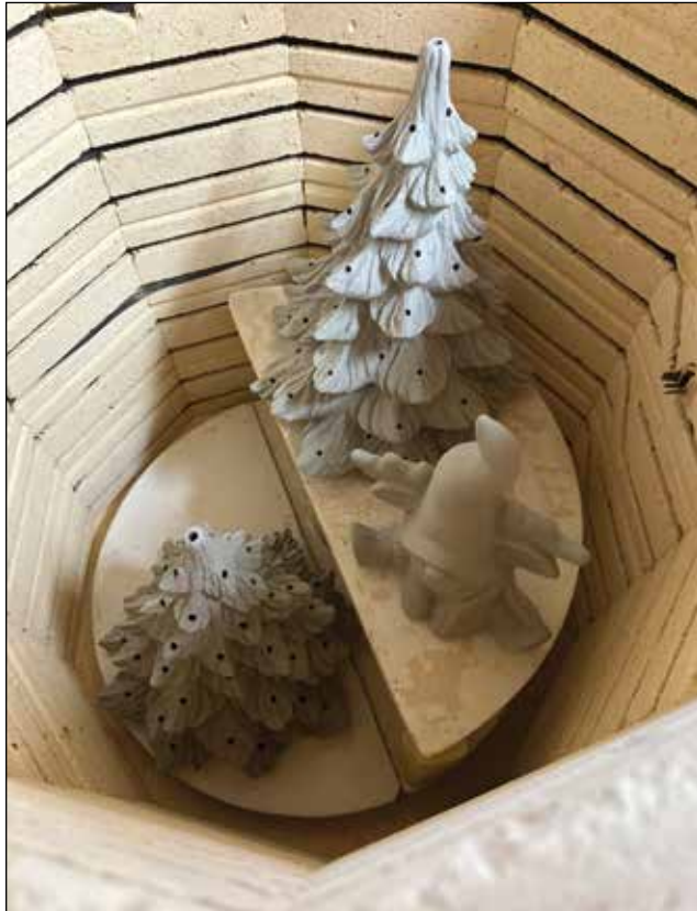
The sanded tree is fired in the kiln, which is opened only after it has cooled completely.
