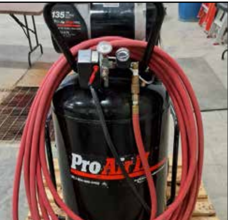
ProAirll Upright Air Compressor w/Cover, 1.7 hp, 135psi, oil free, Model 919. 195411
