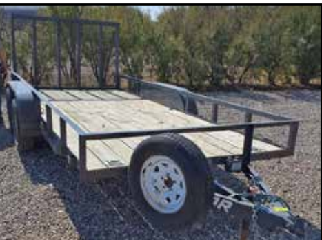
Lamar 16' Flatdeck Bumperpull Trailer, 77" wide deck, 2" ball, 78"wx50"l ramp deck, tire size 75R15, 6 tie down rings
