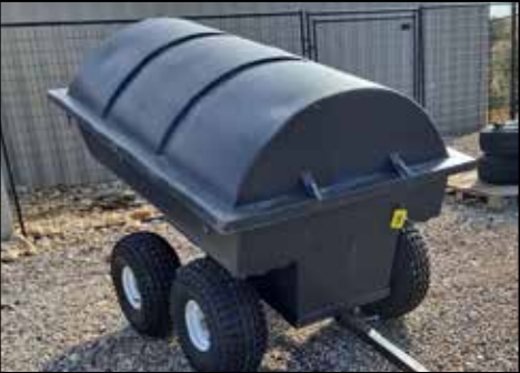
Poly Utility Dump Trailer with Cover, Box size 6'x4', 2 inch ball.
