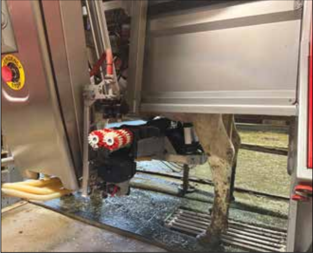
ROBOTIC MILKING: A cow enters the robotic milking station, where cows are milked voluntarily three times a day.
