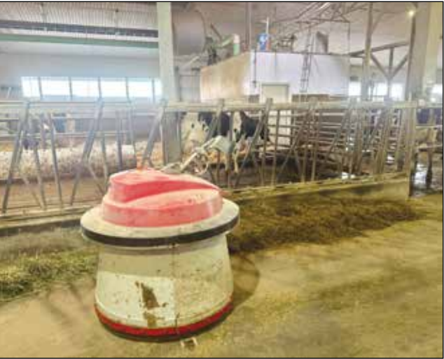
AUTOMATED FEEDING: A robotic feed pusher moves feed closer to the cows every hour throughout the day.
